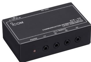
For remote transceiver control using a personal computer equipped with an RS-232C port. You can change frequencies, operating mode, memory channels, etc., via your computer.
