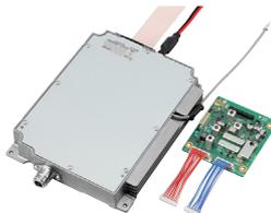
Allows you additional all mode operation on the 1200 MHz frequency band.
